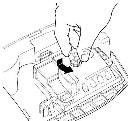
3. For SN6031 and SN6041: unscrew the faulty lamp. Insert a new 230V / 60W lamp with E27 fitting.
